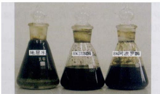
图5 油水混合初期摇匀后的状态 Fig.5 Oil-water state at the initial mixing stage after shaking up
