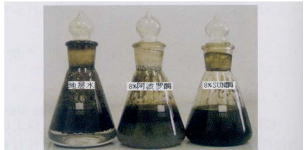
图7 油水混合48h摇匀后的状态 Fig.7 Oil-water state after mixing for 48 h and shaking up
