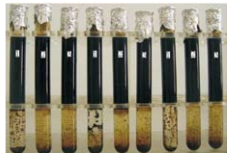
图 3 SUN 酶洗油实验油水混合 48 h 后状态 Fig.3 Oil-water state after mixing for 48h in washing oil experiment with SUN enzyme
